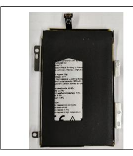
Remove the battery then separate the battery and the battery panel.
