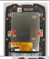
Remove 2 ST1.7\*3.5 screws from the LCD panel, then remove the LCD panel.
