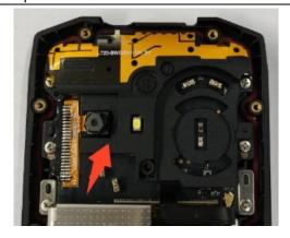
Tilt the camera from the upper Bracket panel so that the camera is detached from the Bracket panel.
