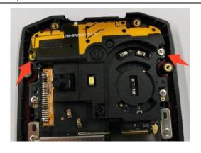
Remove the 2 ST1.7\*3.5 screws and remove the upper bracket.
