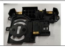
Remove the flash board from the upper bracket panel.
