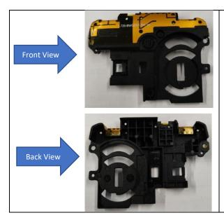
Remove the flash board from the upper bracket panel by Tweezers.
