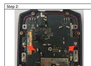
Remove the 2 ST1.7\*3.5 screws that hold the motherboard in place, then remove the motherboard
