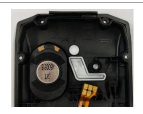
Peel off the double-sided adhesive release paper, put the speaker into the B shell, pay attention to the assembly in place at one time, and press the speaker firmly for 10S clock (50N)
