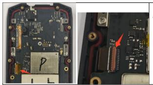
Remove the insulating tape from the connector and open the connector.
