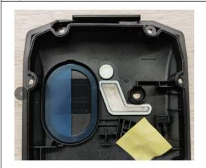
Clean up the adhesive residue and paste the double-sided tape of the speaker.
