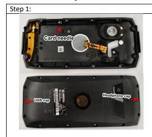
Check that the card needle is in place; Headphone cap is in place; The USB cap is in place
